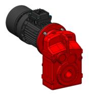
**Craftsman Travel Drives** consist of Parallel shaft helical gearbox and Electric motor which provides efficient and compact solution for Drives. Gears are made of case hardened alloy steel and profile corrected to ensure the maximum transmissible torque, gears and bearing are oil bath or splash lubricated which serve silent operation and improve the reliability of gears. Electric motors are 3 Phase induction type which conforming to latest IEC/IS standards.
